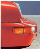
The deformable body panels encase resilient bumpers.
