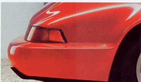
Aerodynamic refinements include deformable front and rear thermoplastic body panels to optimise the airflow and absorb low speed impacts.
