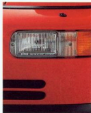
Integral foglamps and indicators are recessed to improve aerodynamics.
