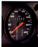
A display in the speedometer indicates the gear and transmission mode.
