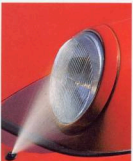
The powerful headlights are kept clean with a high pressure water-jet.
