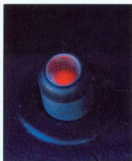
The integral alarm system is automatically armed by the central-locking system.
